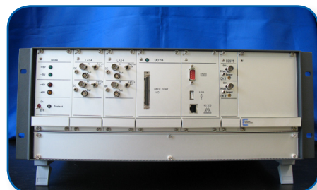
View of rack including a Switching converter SC24, a Linear Amplifier LA24-2, a UC75 real time controller and a Eddy Current Sensor ECS75-2
