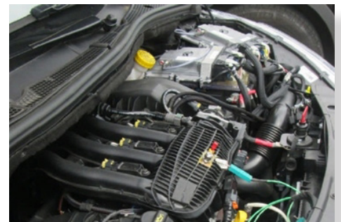
Fig2: e-Lift3 ElectroMagnetic Actuators integrated in a 3-cylinder thermal engine
