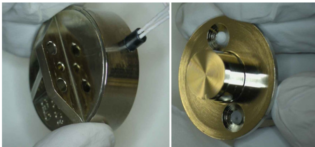
Fig8: Space certified Unlocking ElectroMagnet Actuator
