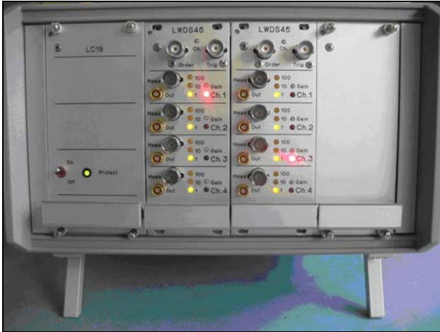
Figure 3.1 Picture of the LWDS45-2, multi-channels drive and sense electronic for piezo-patches.
