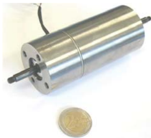
Fig. 5: Damper with a double piston rod
