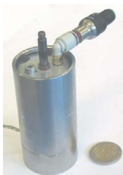
Fig. 2: Damper with a single piston rod
