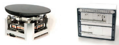
Fig. 7: FSM with non-coated SiC mirror with its customised controller
