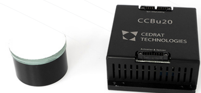
Fig. 11: Fast Steering Mirror with its controller
