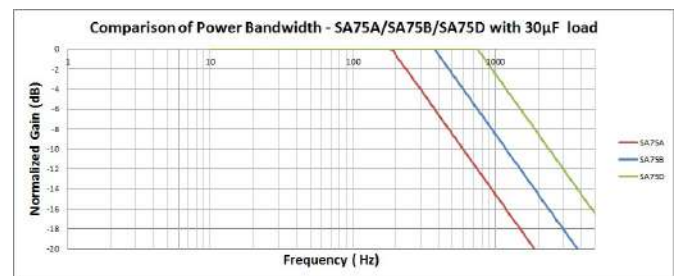
Fig. 8.i: Comparison of power bandwidth for SA75A, B, D for Permanent output current
