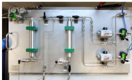
Fig. 3.aa: Bench for testing pressure-regulation piezo valve for ARIANE 6 launcher
