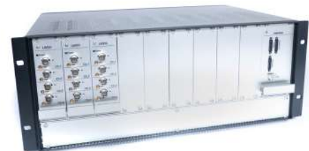
Fig. 9.t: 12 channels emission piezo rack
