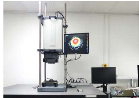
Fig. 1.h: Measurement of the flatness of a FSM mirror using Zygo interferometer
