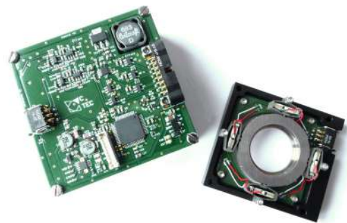
Fig. 7.r: Micro scanning piezo XY stage (+/- 10 \mu\text{m} stroke) and its driver box for image resolution enhancement
