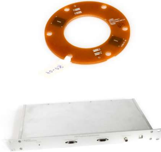
Fig. 9.n: EUCLID-NISP top counter sensor and associated electronics
