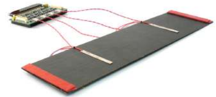
Fig. 9.r: Test bench for SHM : LWDS45 board connected to 2 piezo patches
