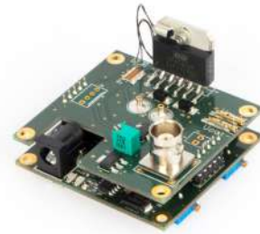
Fig. 8.x: OEM amplifier board for driving magnetic actuators
