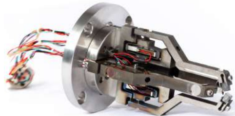
Fig. 7.q: Active slits (> 700 \mu\text{m} aperture) for X ray beam shaper designed with SOLEIL for the SWING beamline
