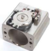
Fig. 5.b: Rotating motor based on MSPA30uXS
