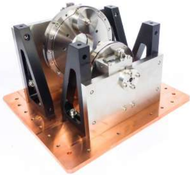
Fig. 5.j: Breadboard models of the gimbal piezo motors.
