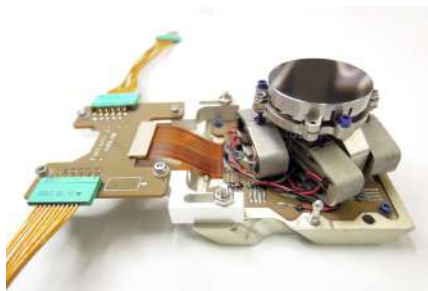
Fig. 3.b: DTT60SM based on 4 APA60SMMSG (courtesy of Airbus DS Sodern)
