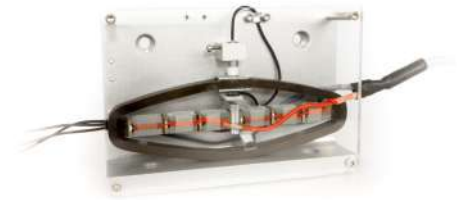
Fig. 4.c: ECP test bench for APA500L-CFRP-ECS
