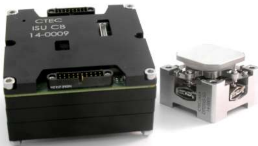
Fig. 7.p: Piezo FSM (+/- 1 mrad stroke) and its controller box for fine laser pointing & stabilization
