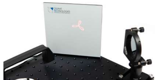
Fig. 7.v: Rosette figure produced by the FSM actuation
