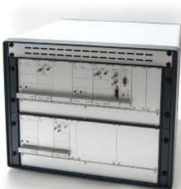
Fig. 8.n: Rack cabinet mounted LA75C push pull amplifier channels for driving large capacitance piezo mechanism
