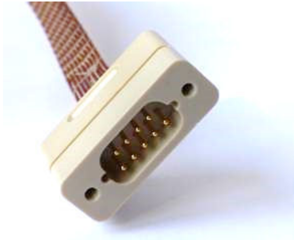
Figure 1 View of output wire of the mechanism with a Male Sub-D 9 connector (High Vacuum compatible).
