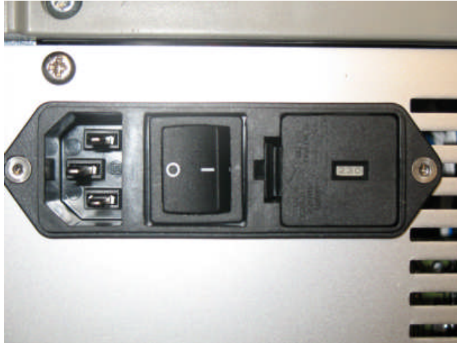
Figure 4: power entry module of the LA75A/ LA75B rack
