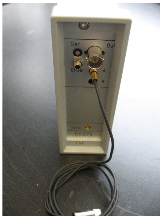
Figure 3-1: Probe connection on the front panel.
