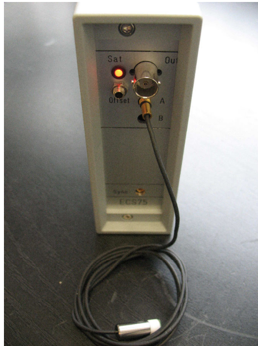
Figure 3-5: Red indicator, sensor is out of range.
