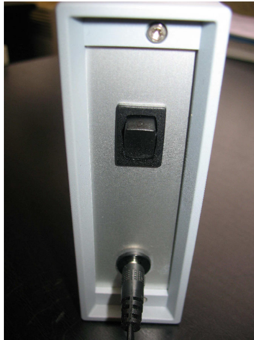
Figure 3-2: AC/DC adapter connection on the rear panel.
