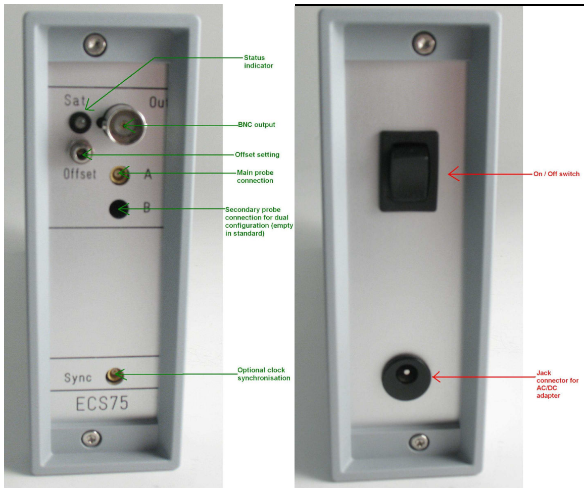
Figure 2-1: Electrical connections of the ECS75 OEM on the rear and front panels.
