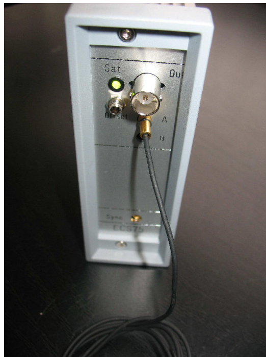
Figure 3-6: Green indicator, sensor is in the range.
