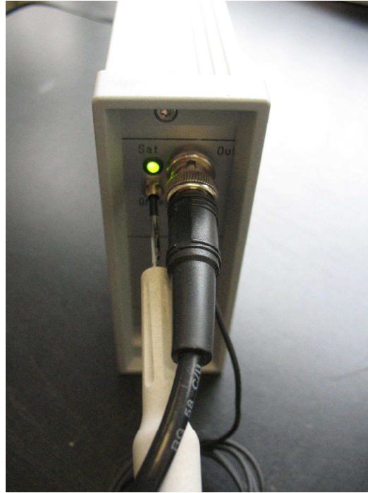
Figure 3-8: Setting the offset of the BNC output.
