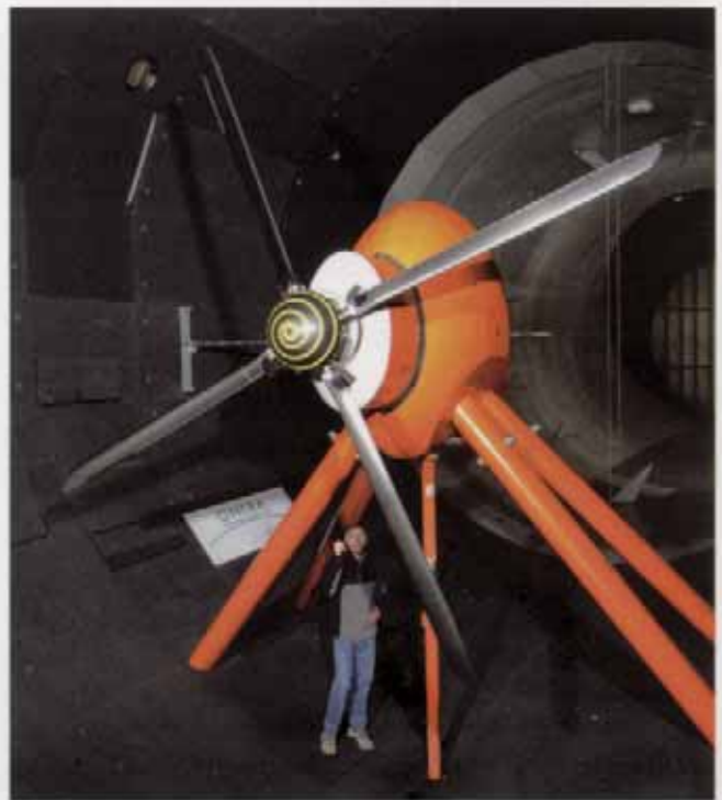
Tests of the active-blade rotor in the S1 wind tunnel at Modane-Avrieux, using trailing edge control flaps; the rotor is 4.2 meters in diameter
