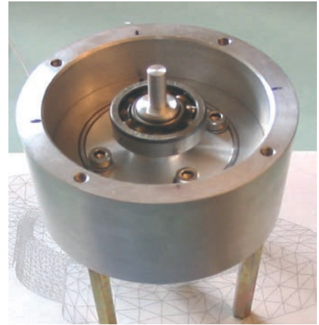
Fig. 5: Frame with rotor and stator
