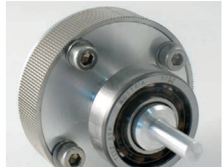
Fig. 6: Shaft with rotor and bearing
