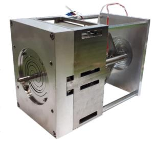
Fig. 1: Inchworm Piezo motor Demonstrator and video
