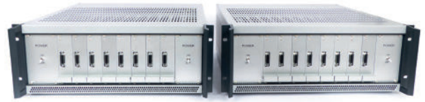
Figure 2: Final 2x48 channels CTEC Drive & Control system
