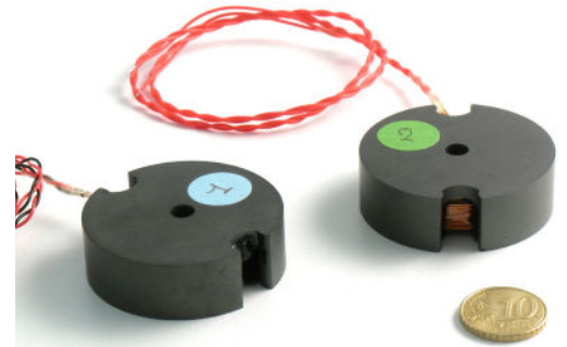
Fig. 1. Magnetic sensors with up to 4cm range
