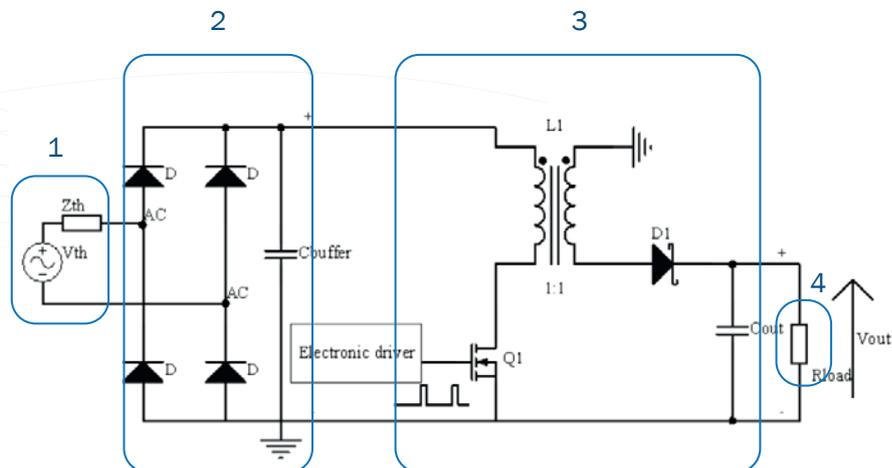
Fig. 3: Schematic view of the AC-DC & DC-DC electronic
