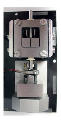
Fig. 1.b: Force and stroke test bench
