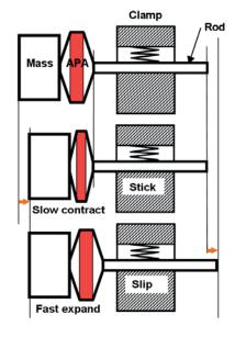
One step of the SPA inertial motor One step realized by two operations:
