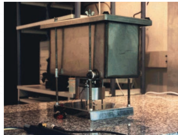
Fig. 3: High power (3kW) magnetostrictive sonar transducer TRIPODE.
