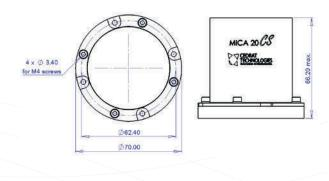
Fig. 3: View of the mechanical interfaces of the MICA20CS proof-mass (MICA20CS actuator + counter-mass + back position sensor)
