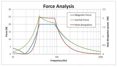
Fig. 4: Force and heat dissipation vs frequency
