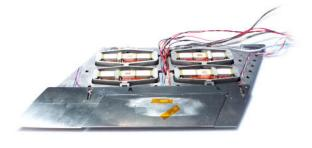
Fig. 6: Overview of the two aileron piezo actuators, integrated into the wing
