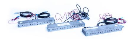
Fig. 3: Overview of 3 PJA after mounting and testing, ready to be implemented into the wind tunnel
