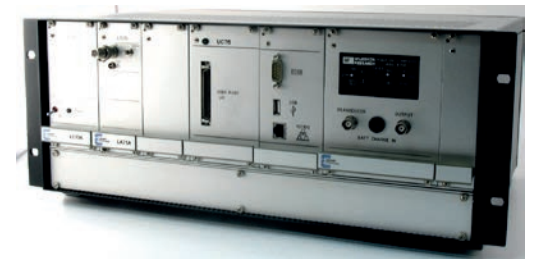
Fig. 5: Human Machine Interface with LabView® software and rack84F including a Unit Control UC75 based on CompactRIO product
