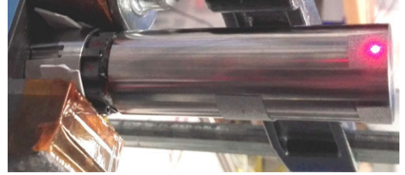
Fig. 4: Piezo actuators factory verification using laser instrument
