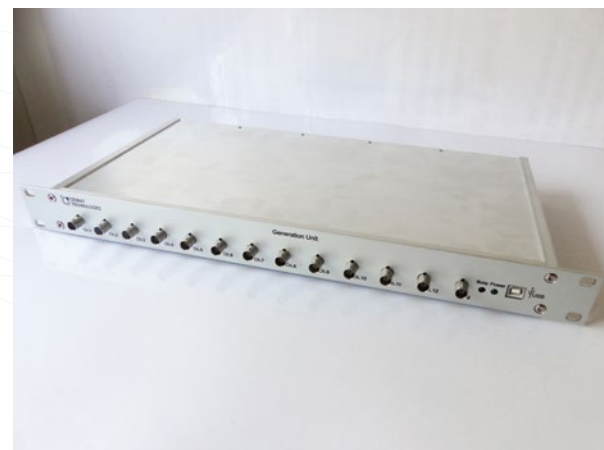
Fig. 8: 12-channel arbitrary generator with 10MSps sampling rate and 14bits resolution and dedicated GUI for configuration.
