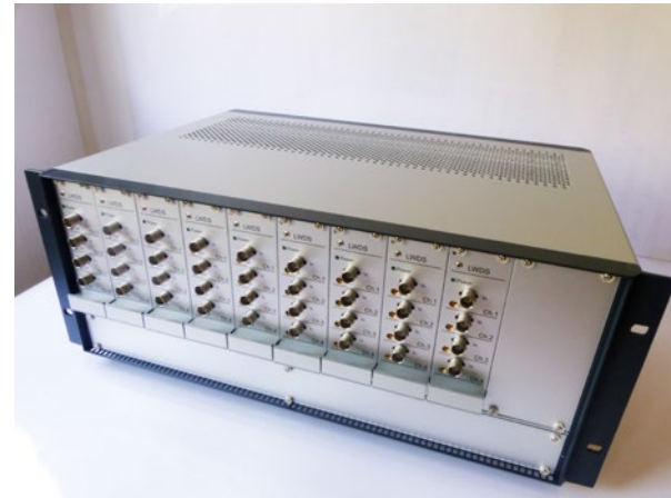
Fig. 6: 36-channel emission unit with \pm 15V output voltage for applications in the 100-1000kHz range
