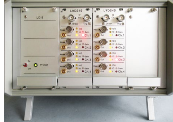
Fig. 1: 8-channel laboratory rack with fully featured SHM channels (DC power supply, emission, reception)
