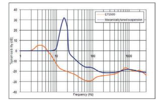
Fig. 2: Comparison of the Electrically Tuneable Suspension performances compared to a conventional passive mechanically tuned suspension performances.
