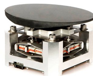
Fig. 18 : FSM with non-coated SiC mirror
