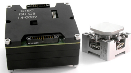
Fig. 6 : DTT15XS-SG with CCBu20 controller
