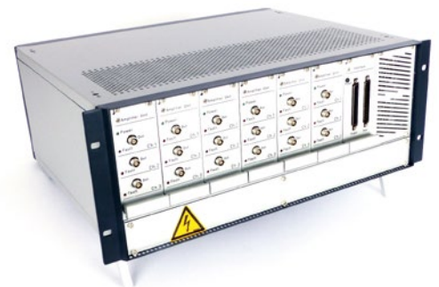
Fig. 7: 18-channel emission unit with \pm 200V output voltage for applications in the 25-40kHz range
