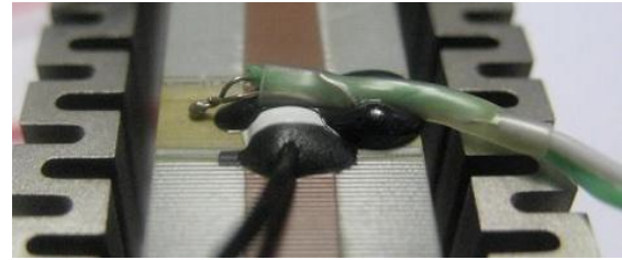
Fig. 6: View of thermocouple attached to the piezoelectric ceramics.
