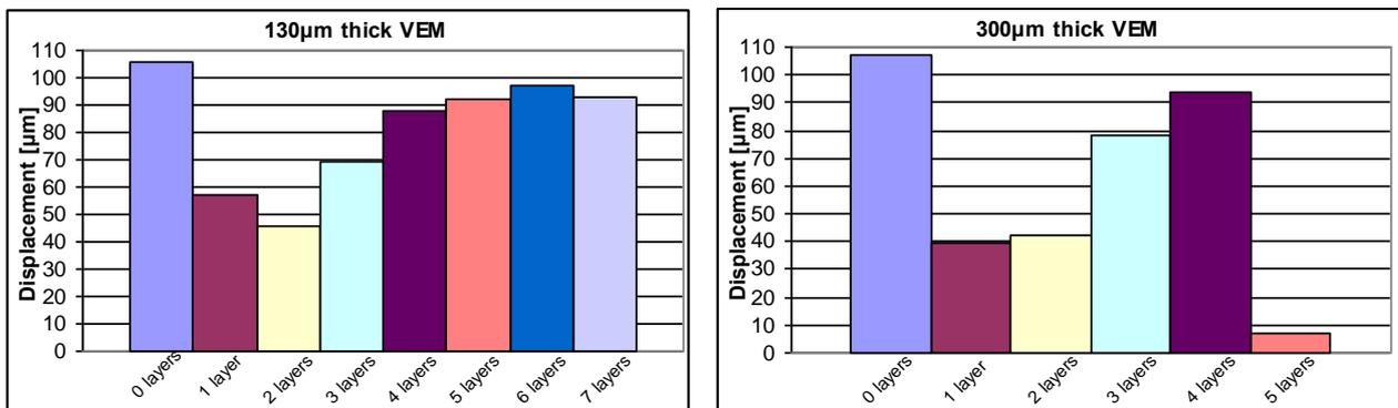
Fig. 8. Stroke measurement for  $130\mu m$  (to the left) and  $300\mu m$  (to the right) thick VEM
