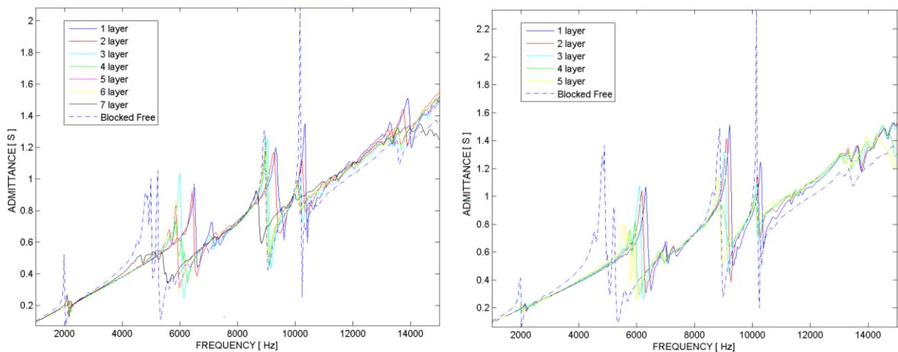
Fig. 9. Admittance curves for 130 $\mu\text{m}$  (to the left) and 300 $\mu\text{m}$  (to the right) thick VEM
