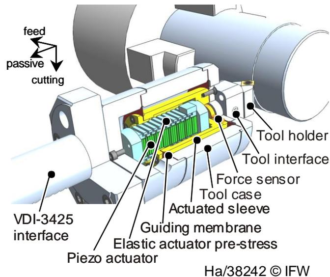
Fig. 2. Active tool adaptor based on PPA®
