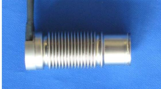
Fig. 5. Custom made piezoelectric ceramics
