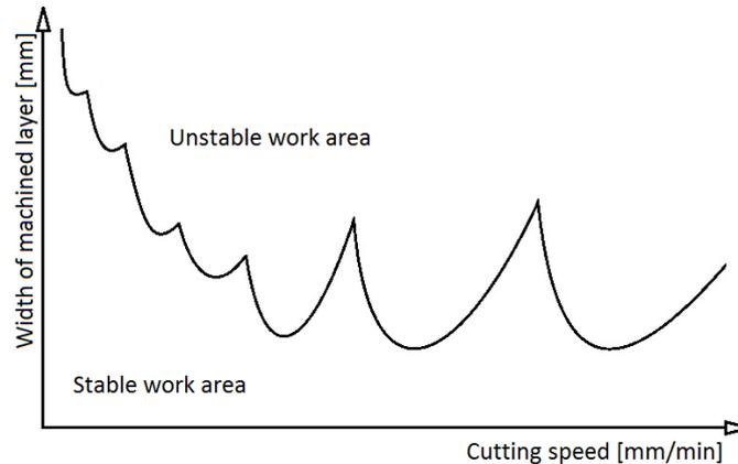
Fig. 1. Stability lobe diagram of typical machine tool
