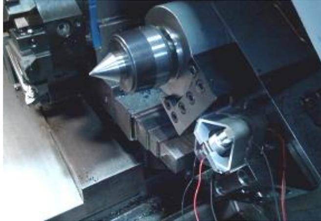
Fig. 13. Location of the APA® on the tailstock
