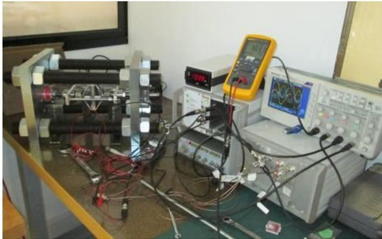
Fig. 11. Blocked force test bench
