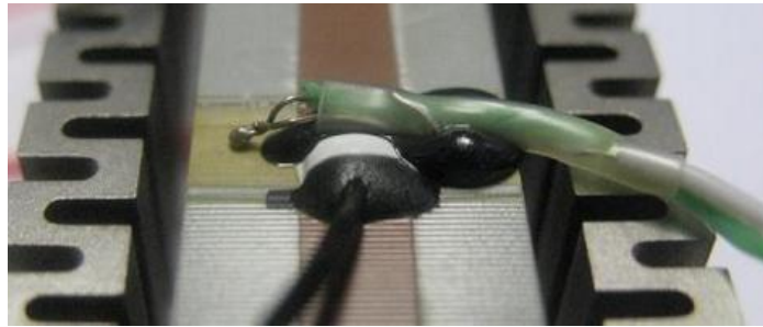
Figure 3: View of thermocouple attached to the piezoelectric ceramics used for temperature measurement.
