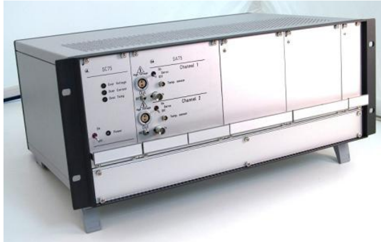
Figure 7: SA75D assembled in standard 19 inches rack.
