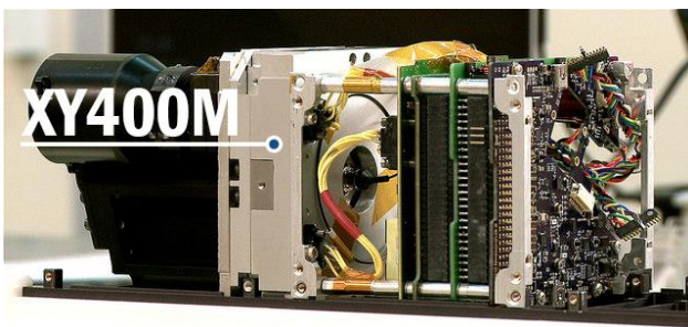
Figure 2: XY400M CTEC product mounted on PicSat
